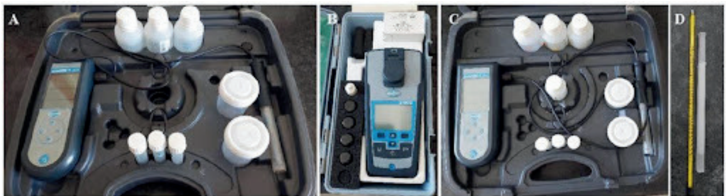
Fig. 3. Different types of handheld sensors for testing aquaculture physiochemical parameters. (A) Conductivity/TDS meter, (B) Digital nephlo-turbidity meter, (C) pH meter, and (D) Scientific thermometer.
